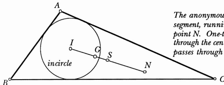
*The anonymous (but herein-dubbed "Nagel") segment, running from the incenter  $I$  to the Nagel point  $N$ . One-third of the way along, it passes through the centroid  $G$ , and halfway along, it passes through the Spieker circle's center  $S$ .*
